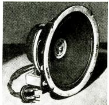
The "6 in. speaker" in the List of Parts. A plug and 24 in. cord are provided.
